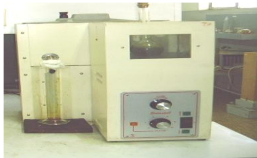
Fig. 8. distillation apparatus for petroleum products.
