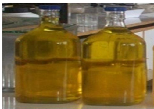
Fig. 6. Jatropha biodiesel after trans-esterification process.
