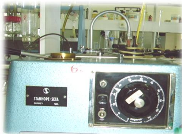
Fig. 10. Pensky martens closed cup flash point tester.
