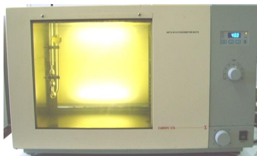
Fig. 7. Cannon-Fenske glass capillary Viscometer apparatus.
