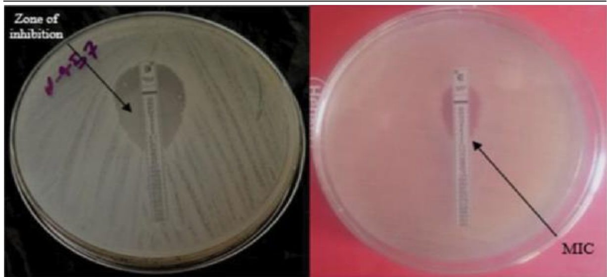
Figure 2. Epsilometry Test E-test inhibition ellipse showing the MIC at the intersection of the growth of the organism
