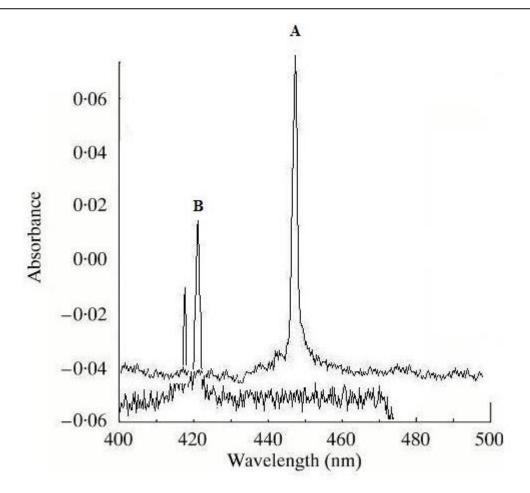
Figure 5. The difference between the optical absorption reductions of the enzyme is attached to the carbon monoxide complex (A) and reduced enzyme as reference (B).
