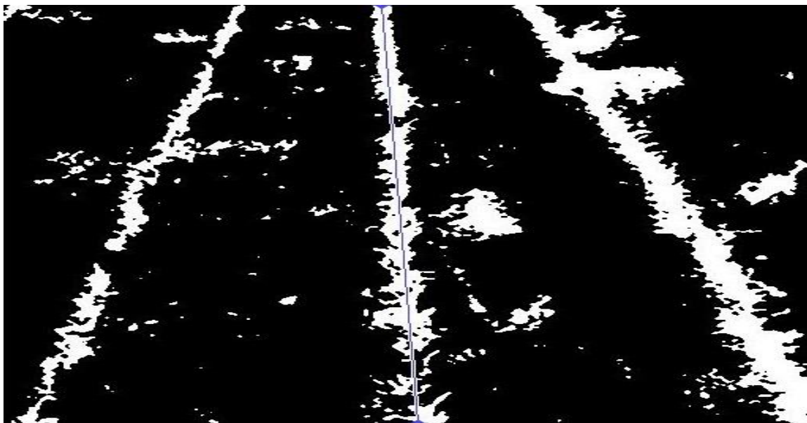
Figure 7 . Detected row by hough transform
