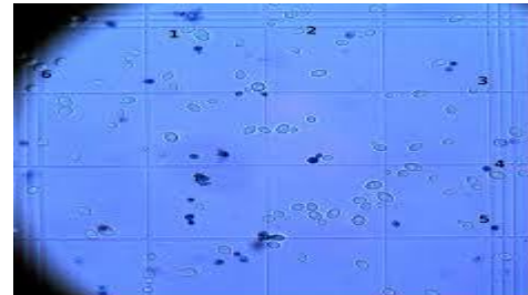
Fig. 2 -acterial colony count by using neubauer slide
